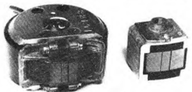
Fig. 7. Double slit ferrite erase head (left), and double system ferrite erase head (right), for studio machines
