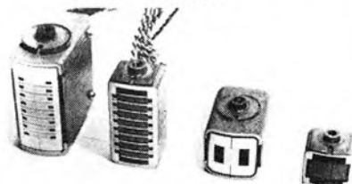
Fig. 8. From left to right. Multi-track playback head unit with eight tracks to one inch; studio playback double system erase head with eight tracks to one inch; Studio playback head with clamp fitting; and double system erase head
